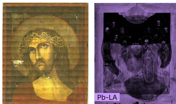
Figure 1: The Pb La intensity distribution map (right) reveals the presence of an older painting that lies beneath the image of Jesus Christ wearing a crown of thorns (left).
