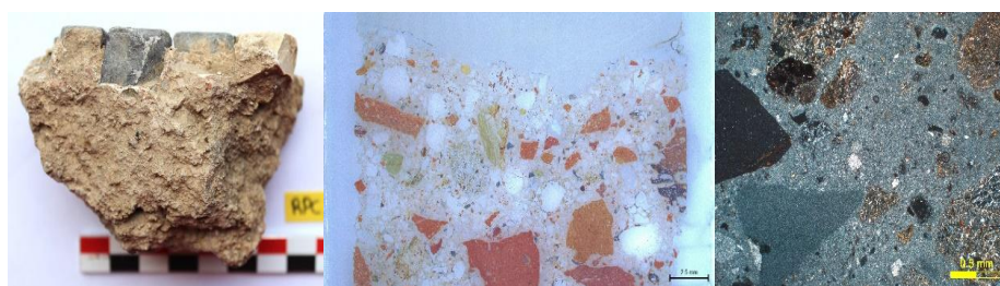
Mosaic supporting layer mortar sample (left). Two images of microscopic techniques investigation.
