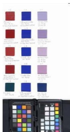
Fig.1a One of the prototype panels containing mixtures of red and blue pigments
